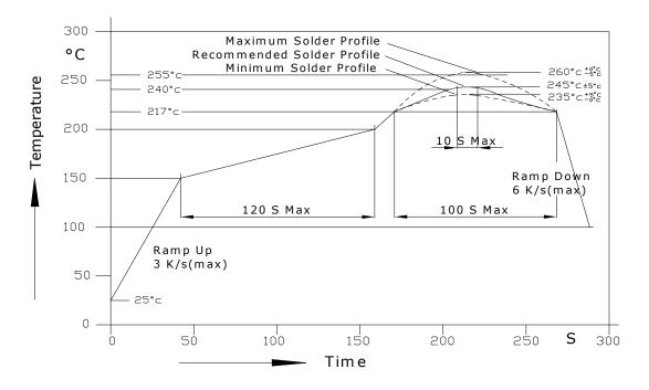
3.2. Reflow soldering should not be done more than two times.
