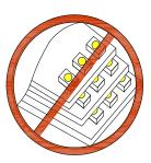
Compare to epoxy encapsulant that is hard and brittle, silicone is softer and flexible. Although its characteristic significantly reduces thermal stress, it is more susceptible to damage by external mechanical force. As a result, special handling precautions need to be observed during assembly using silicone encapsulated LED products. Failure to comply might lead to damage and premature failure of the LED.
