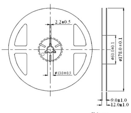
Unit: mm Tolerance:  $\pm 0.25$ mm
