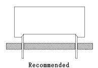
The component shall be placed at least 5mm from edge of PCB to avoid damage caused excessive heat during wave soldering.
