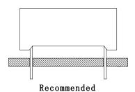
The component shall be placed at least 5mm from edge of PCB to avoid damage caused excessive heat during wave soldering.
