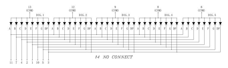
Internal Circuit Diagram (Common Cathode)
