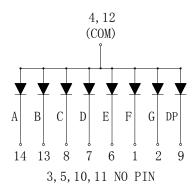
Internal Circuit Diagram (Common Cathode)
