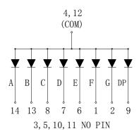
Internal Circuit Diagram (Common Cathode)
