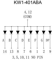
Internal Circuit Diagram (Common Cathode)
