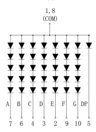
Internal Circuit Diagram (Common Cathode)
