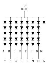
Internal Circuit Diagram (Common Cathode)
