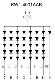
Internal Circuit Diagram (Common Cathode)
