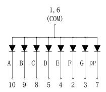
Internal Circuit Diagram (Common Cathode)
