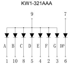
Internal Circuit Diagram (Common Cathode)
