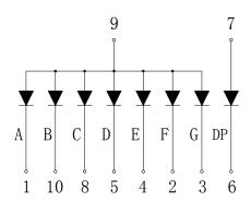
Internal Circuit Diagram (Common Cathode)
