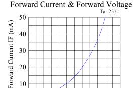
) 5.4 5.8 6.2 6.4 6 Forward Voltage VF (V)
