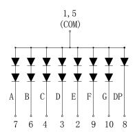
Internal Circuit Diagram (Common Cathode)
