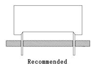
3. The component shall be placed at least 5mm from edge of PCB to avoid damage caused excessive heat during wave soldering.
