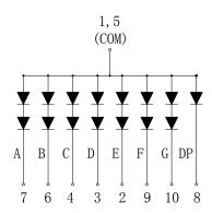
Internal Circuit Diagram (Common Cathode)
