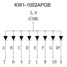
Internal Circuit Diagram (Common Cathode)
