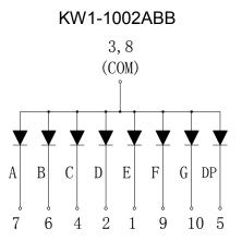
Internal Circuit Diagram (Common Cathode)
