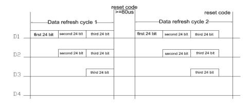
Note: The data of D1 is send by MCU, and D2, D3, D4 through pixel internal reshaping amplification to transmit.
